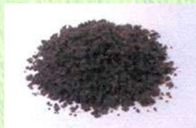
Water-cooled slag forms sand
