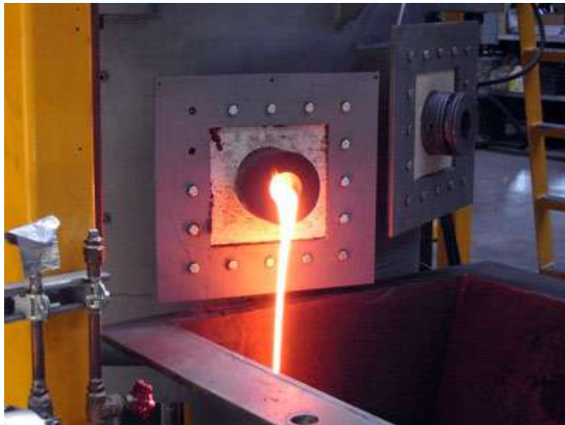
Molten slag draining from a plasma furnace
